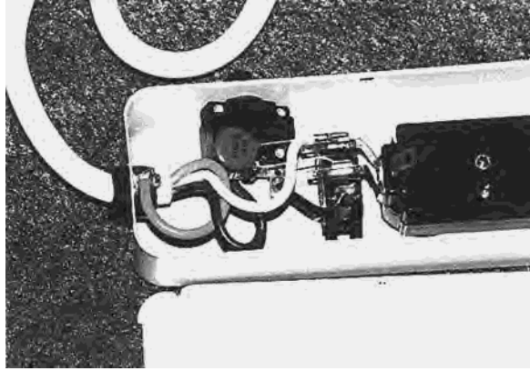
Figure 11-3—Disassembled surge suppressor
